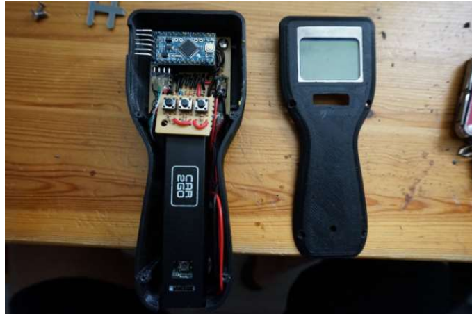
Figure 15: Assembly of the USB battery pack, LCD, and faceplate
